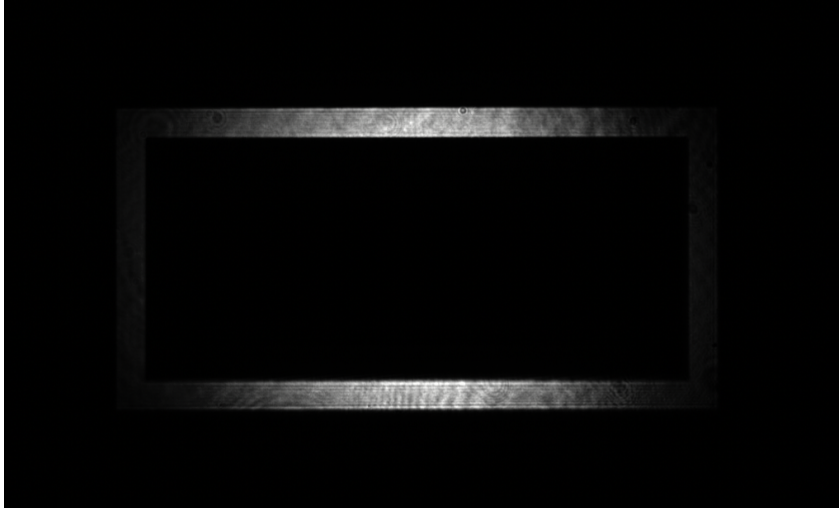
Figure 3.7: Grayscale image of a box made by the DMD with a gaussian input beam, taken by a ThorLabs CMOS camera. The light intensity varies and decrease rapidly for the long side.
