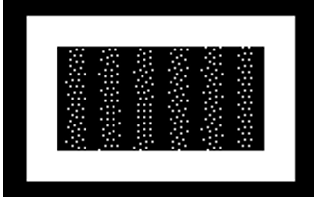
Figure 3.17: Binary pattern of the sinusoidal perturbation with six spatial periods, generated by the “JarvisHalftone” error diffusion method.
